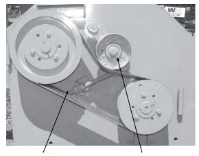
Idler Adjusting Rod Idler Pulley
