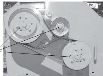
2. Clean any clippings from gearbox areas, pulley areas and anywhere else that is prone to excessive heat where fires can start.
