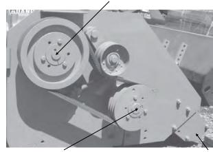
2 Main Cutter Drum Bearings (One on each side behind pulley)
