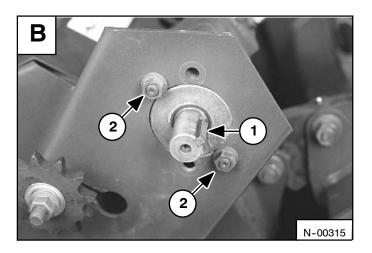
Remove the key (Item 1) [B] from the drive motor shaft.
