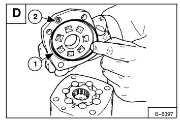
Remove the valve plate [D].
