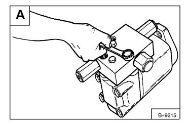
Remove both relief valves from the port block [B] & [C].
