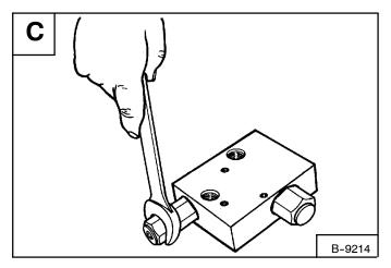
Remove the flow divider valve [D].
