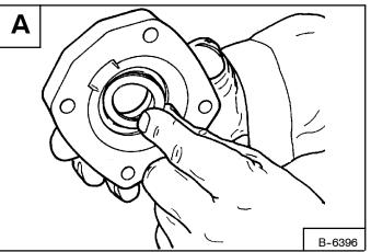
Remove the shaft and bearing assembly from the housing **[B]**.
