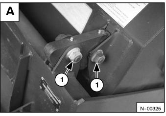
Remove the hinge bolts (both hinges) [B].
