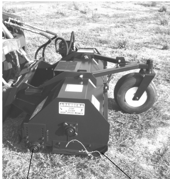
Gauge Roller Running on Ground
