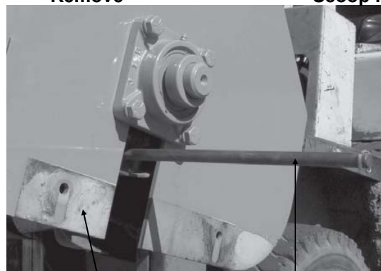
Skid Shoe Area
