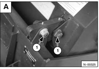
Remove the hinge bolts (both hinges) [B].
