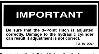
Do not adjust the 3-Point Hitch so that the lower points of the 3-Point arms go *over center* [C] & [D].
