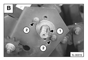
Remove the key (Item 1) [B] from the drive motor shaft.
