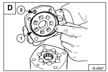
Remove the valve plate [D].
