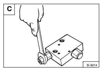
Remove the flow divider valve [D].
