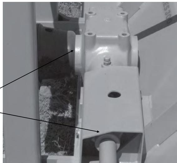
3. Clean the inside of the mower with a pressure washer. Make sure the inside of the mower is kept free from mud and compact grass. Keep in mind that mud built up on the cutter drum can cause imbalance.
