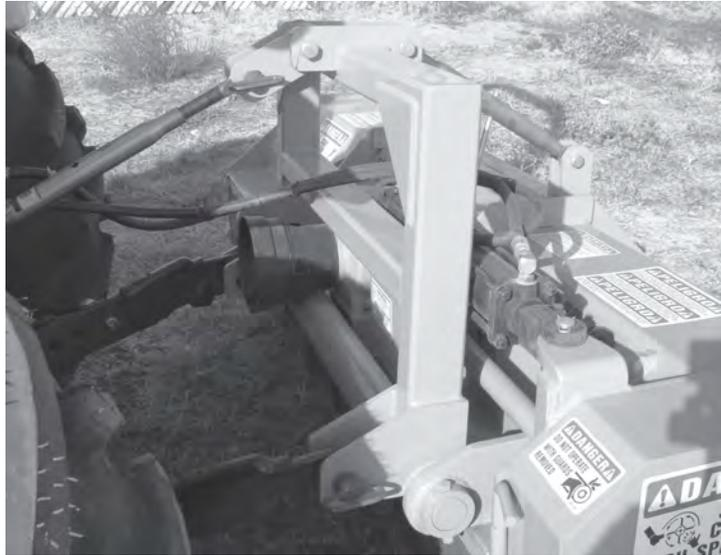
1. Back the tractor so the lift links are in-line with the mower's hitch pins.
