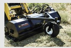
The F-Series can include a **front-mounted**, **foam-filled caster wheel** to adjust cutting height, ensuring smooth operation on diverse terrains.
