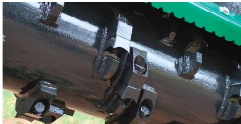
The FX36 is equipped with 2" Quadco Knives, designed for enhanced cutting strength and durability, ideal for tackling tougher vegetation.
