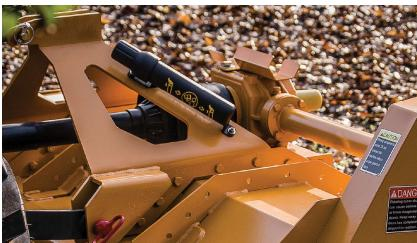
Adjustable Cat-1 hitch allows center-mounting or **6-inch offset**, enhancing versatility for mowing around obstacles and structures.
