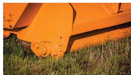
Adjustable rear roller with a range of **0 to 3.5 inches**, providing versatile cutting heights.
