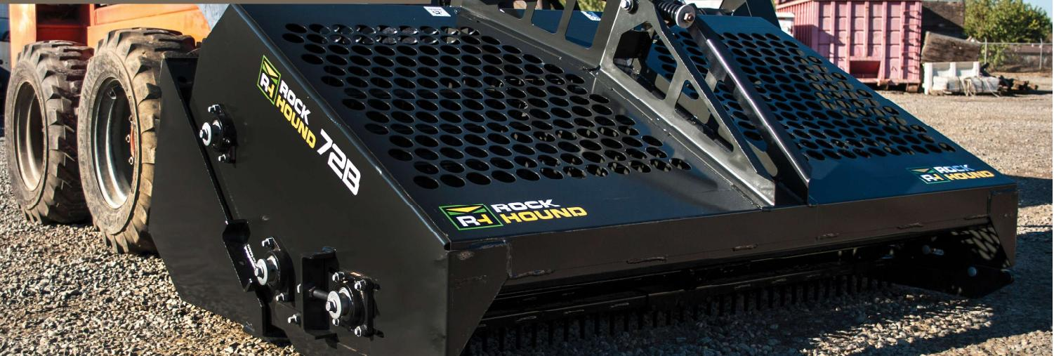
The Rockhound 72B Landscape rake is the original skid steer implement designed to **remove rocks, level ground before sod is laid or prepare seedbeds**. It was one of the first five Bobcat® attachments more than 40 years ago. It eliminates hand raking and picks up rocks as small as 3/4" as well as most rocks up to 8". An optional adapter plate allows the Rockhound 72B-3 Landscape rake to be hooked up to a tractor with a 3-point hitch.
